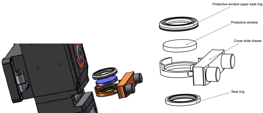
Figure 12. Protective windows of focus lens.
